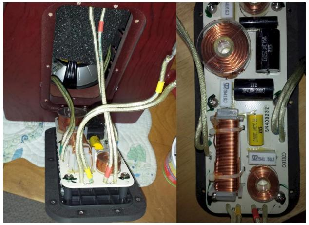
I stripped all the parts off the board except for two of the inductors, and then relocated one inductor, changed the other iron core inductor to air core, and replaced all the resistors and capacitors, so didn't save much by using the old board...
